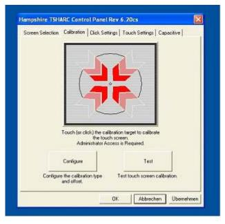
3. Select [Configure] to set up calibration
